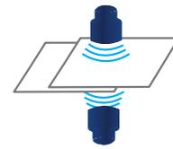
**Ultrasonic Multi-Feed Detection:** To prevent more than one document being scanned at one time the ADS-2100 uses ultrasonic multifeed detection that ensures no documents are missed.
